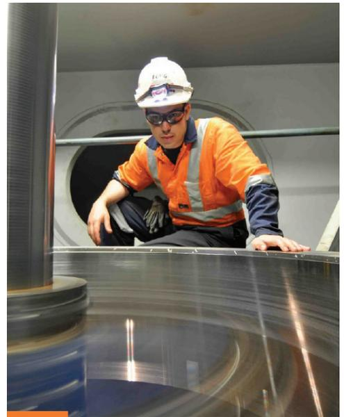
The survey results are analyzed to determine the minimum error envelope achieved. Written reports display the original data, the error from the plane of best fit and total flatness envelope.
