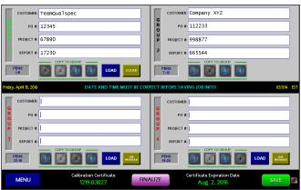
**Job Information:** Job information is entered per group of six inputs to facilitate data entry and traceability. Information can be entered manually, recalled from the previous job, loaded from a text file or copied directly from one group to another which reduces time and entry errors.
