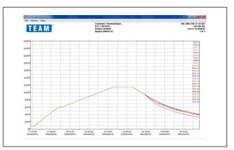
**Trend Chart:** Printed charts can be configured with multiple options including orientation, time interval and which pens to display. The hard-coded job information in the header ensures data integrity for traceability of performed jobs.
