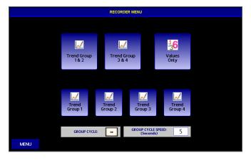
**Recorder Menu:** There are several options for viewing temperature data that can be set per the user's preference and needs. The system can scroll through trend screens at a set pace or view temperature values for all zones at a glance.
